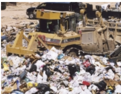
The D7R at Grey Wolf does a great job moving trash, but it's no good as a compactor.
